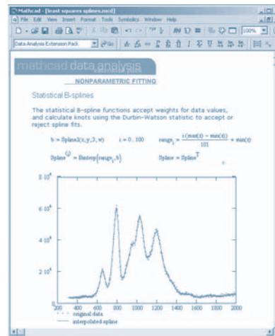
New least-squares B-splines offer optimal compression of data while retaining all significant features of the dataset.
